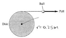
produces a linear acceleration of the ball that obeys the equation a(t)=At, where t is in seconds and A is a constant. The cylinder starts from rest, at t=3.00 s, the ball's acceleration is a=1.80 m/s<sup>2</sup>.
