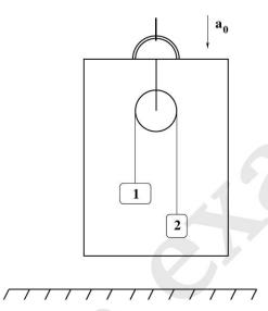
An Atwood machine consists of two massive blocks  $(m_1 \text{ and } m_2)$  tied to the ends of a massless rope that is draped over a massless pulley, as shown. The massless pulley is, in turn, suspended by a second rope from the roof of an elevator that is accelerating downward with a magnitude  $|\vec{a}| = a_0$ .
