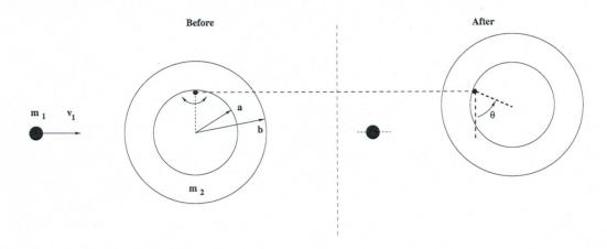
5) A uniform washer of mass  $m_2$ , inner-radius a and outer-radius b is attached to an axle so that it is free to rotate in the vertical plane. The rotational inertia of the washer **about its center-of-mass** is given by  $I_{cm} = \frac{1}{2}m_2(a^2 + b^2)$ .
