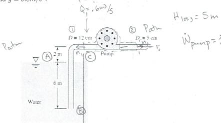
$$V_2 = \frac{Q_1}{A_2} = \frac{.6m^3/s}{\pm (.05)^2} = 305.58 \text{ m/s}$$
