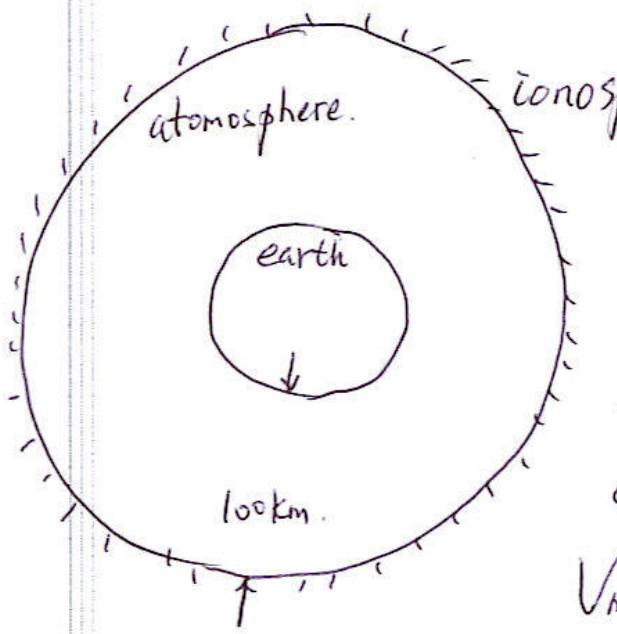
This value of the potential assumes that the radius of the outer concentric conducting sphere is infinitely far away. In fact, the ionosphere above the earth is only 100 km away.
