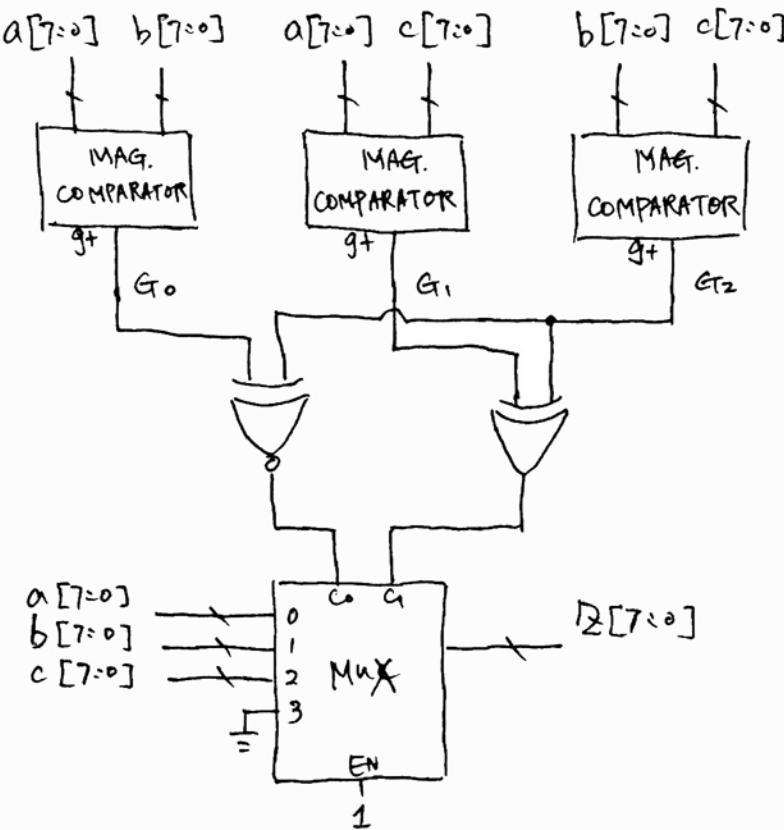
Magnitude Comparator will take in 2 8-bit inputs & output true if  $a > b$ .
