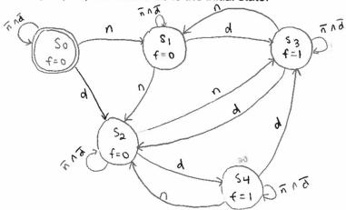
(b) Fill in a state transition table for 2 of the states, S0, the initial state, and a state that produces an output f. If you have more than one state that produces an output, choose one (Sx where x can be whatever you chose in your numbering). You don't need to use all the lines in the table below.
