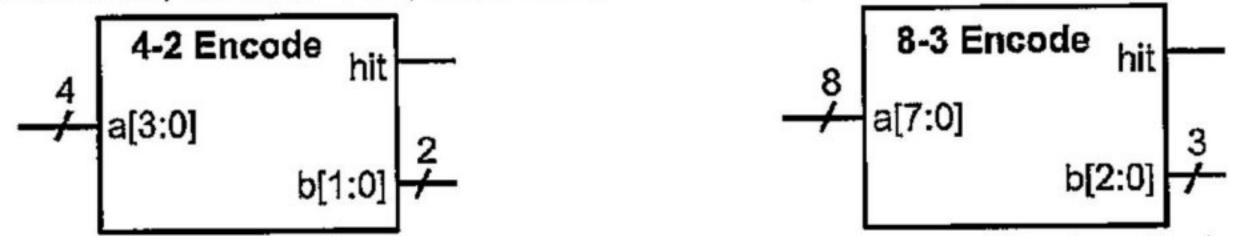
(a) Use instances of this 4-to-2 encoder block to design an 8-to-3 encoder. On-hot inputs are a[7:0], binary outputs are b[2:0], and a hit indicator. You may use additional OR, AND, or Inverters as needed but use as few as possible.
