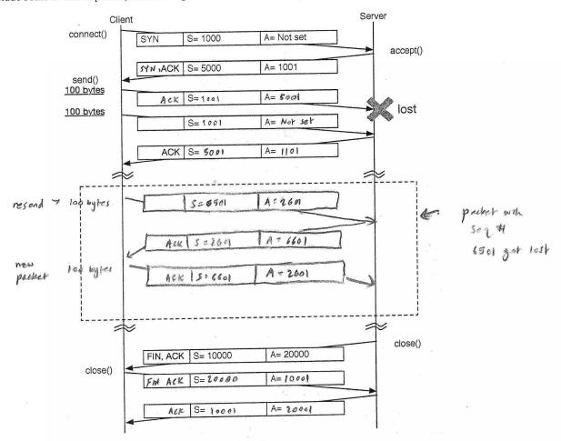
4.1 (10 points) In the figure above, fill in all the missing values for sequence, acknowledgement numbers and flags (SYN, ACK, FIN). For acknowledgement number write "Not set" if acknowledgment flag not set.
