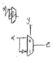
UCLA | EEM16/CSM51A | Spring 2018 (e) (3) A designer modified the basic DFF as shown below to make a GDFF where the clock signal is ANDed with an Enable signal. This approach is known as "clock gating". How does the GDFF's characteristics compare to that of the DFF? Select the answer.
