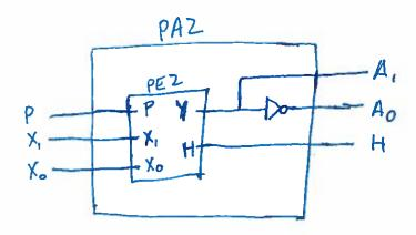
5.0(g). Use two PA2 blocks, plus any CMOS gates or muxes, to generate the PA4 block, which is the privileged arbiter generating an m=4 bit one-hot output A and a one bit output H from m=4 bit input X and one bit input P. (3pts)
