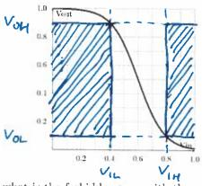
1.6(a). If  $V_{OL}$ =0.1 and  $V_{OH}$ =0.9, what is the forbidden zone with the smallest width that we could set for  $V_{in}$ ?
