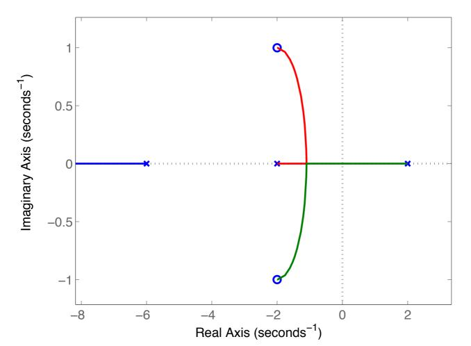
2. No overshoot => no complex poles All poles are real => All components of time domain response are of form e-ot For rise time, Settling time is dominated by the component with smallest [o] .: Best operating point is the break-out point. 3. Consider the C.E in the form a(s) + kb(s) = 0 at s = -1: ie.s3 + (k+6) 52 + (4k-4) 5 + 5k-24 =0 at s=-1 (1 - 1 + (k+6) = -(4k-4) + 5k-24 = 0: 2k -15 = 0 .. K = 15
