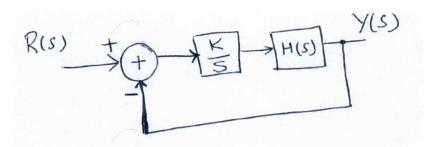
What is the steady state error now if the input is a step function?
