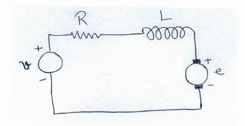
Consider the above circuit representing a DC motor being driven by a voltage source.
