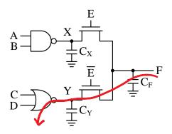
The discharging path goes through  $\overline{E}$ -controlled and C-controlled NMOS transistors. So the pull-down resistance is:
