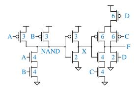
(c) Calculate the switching probability  $\alpha_{0\to 1}$  at *X* and *F* if all inputs have a probability of logic "1" equal to 0.5, i.e. p(A=1) = p(B=1) = p(C=1) = p(D=1) = 0.5. (4 pts)
