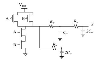
In the circuit shown above, a 2-input NAND gate drives an interconnect, which is modeled by the RC network connected to the NAND gate as shown. Calculate  $\tau_{HL}$  from A to Y when B = 1 and A = 0  $\rightarrow$  1. Also calculate  $\tau_{HL}$  from B to Y when A = 1 and B = 0  $\rightarrow$  1. Are the two time constants different? Briefly (in one sentence) explain why. NMOS transistors have shared diffusion.
