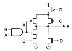
For this question assume a unit inverter of size  $W_p = 3\mu m$ ,  $W_n = 2\mu m$ ,  $R_N = R_P = R_0$ for the unit inverter, and  $C'_{gate} = 2\frac{fF}{\mu m}$ ,  $C'_{diffusion} = 1.5\frac{fF}{\mu m}$  for individual transistors (per  $\mu$ m of transistor width). Assume  $V_{DD} = 1V$  and clock frequency of 1GHz.
