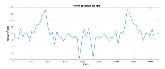
Clearly the above spectral representation leaves much to be desired and one would have a hard time identifying the two tones in the signal.
