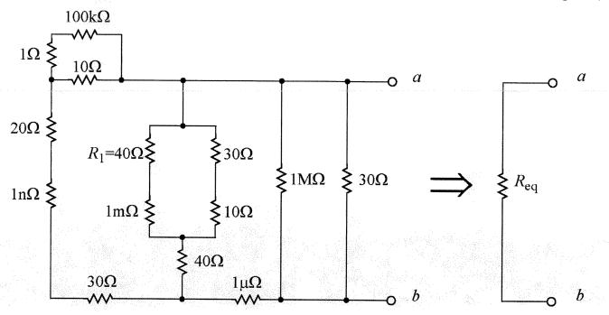
1-1. Reduce the following resistor network to single resistor and find its approximate value (i.e., to two significant digits). Show your work in order to receive full and partial credit. Draw intermediate circuit diagrams as you simplify the resistor network.
