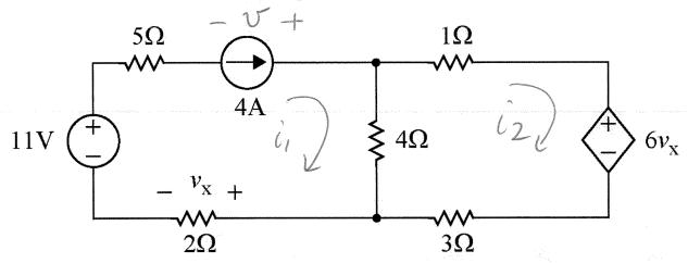
3-1. Calculate the power in each of the 8 components, and state whether it is generating or absorbing power. Show all intermediate calculations to receive full and partial credit.
