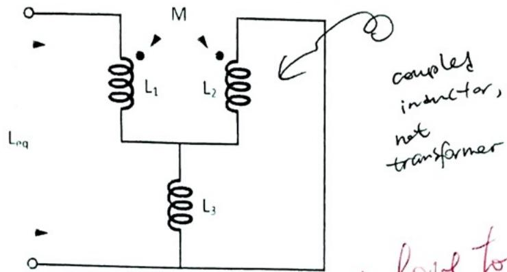
$$\left\{ \begin{array}{l} V_1 = L_1 \frac{di_1}{dt} + M \frac{di_2}{dt} \\ i_2 = L_2 \frac{di_2}{dt} + M \frac{di_1}{dt} \end{array} \right.$$
