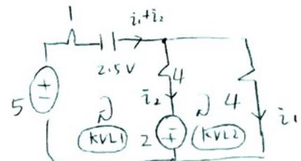
$$\left. \begin{array}{l} -2.5 - 4i_2 + 2 + 5 - i_1 - i_2 = 0 \\ -2 + i_2 \times 4 - 4i_1 = 0 \end{array} \right\} (KVL1)$$
