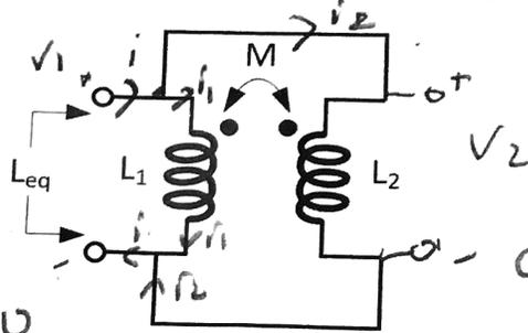
$M$  should be added since currents enter inductors through dots.
