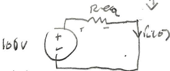
By KVL, voltage across the resistor = 100V
