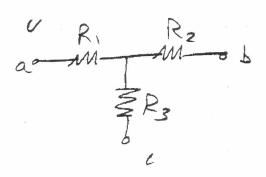
$$R_{4} = \frac{R_{1}R_{2} + R_{2}R_{3} + R_{3}R_{1}}{R_{1}}$$
