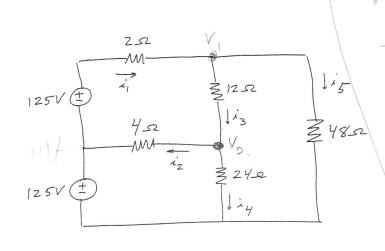
$$\frac{V_1 - 105}{2} + \frac{V_1 - V_2}{12} + \frac{V_1 + 125}{48} = 0.$$
