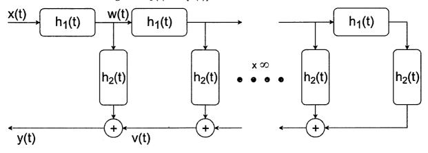
(a) (8 points) In terms of  $H_1(s)$  and  $H_2(s)$ , what is the equivalent transfer function  $H_{eq}(s)$  between Y(s) and X(s)? Hint: how does  $\frac{V(s)}{W(s)}$  relate to  $\frac{Y(s)}{X(s)}$ ?
