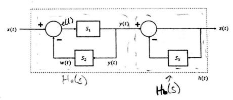
(a) (8 pts) Compute the IRF of entire system h(t) and its Laplace transform H(s).
