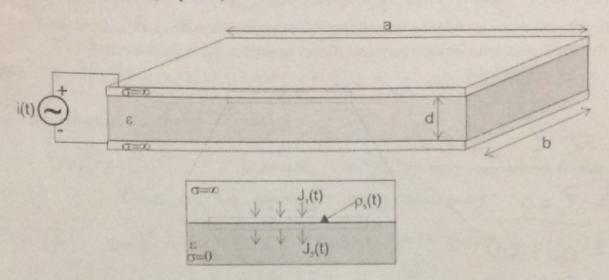
(a) (15 points) Consider a parallel plate capacitor with plate dimensions a and b, and a perfectly insulating dielectric of thickness d, and a permittivity  $\varepsilon$ . Assume that the capacitor is hooked up to a current source with time varying current  $i(t)=i_0\cos(\omega t)$ . The voltage difference between the plates is v(t). The capacitor obeys the standard relation  $i(t) = C \frac{dv(t)}{dt}$ .
