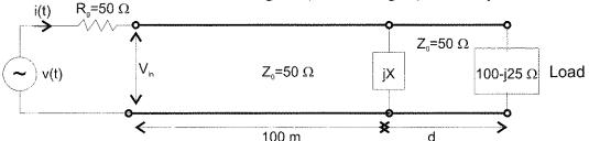
Since the matching element is a shunt, it makes more sense to work with admittance. YL= 0.47+j 0.12
