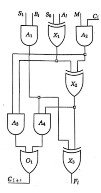
Determine the switching expressions for the outputs  $F_i$  and  $C_{i+1}$ . Using AND, OR, NOT, XOR expressions as appropriate fill in the following table:
