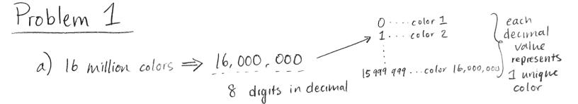
We need to represent 8 digits in BCD code. BCD code requires 4 bits to represent 1 digit in decimal. Thus, we need 4x8=32 total bits to encode the color spectrum of 16,000,000 colors.
