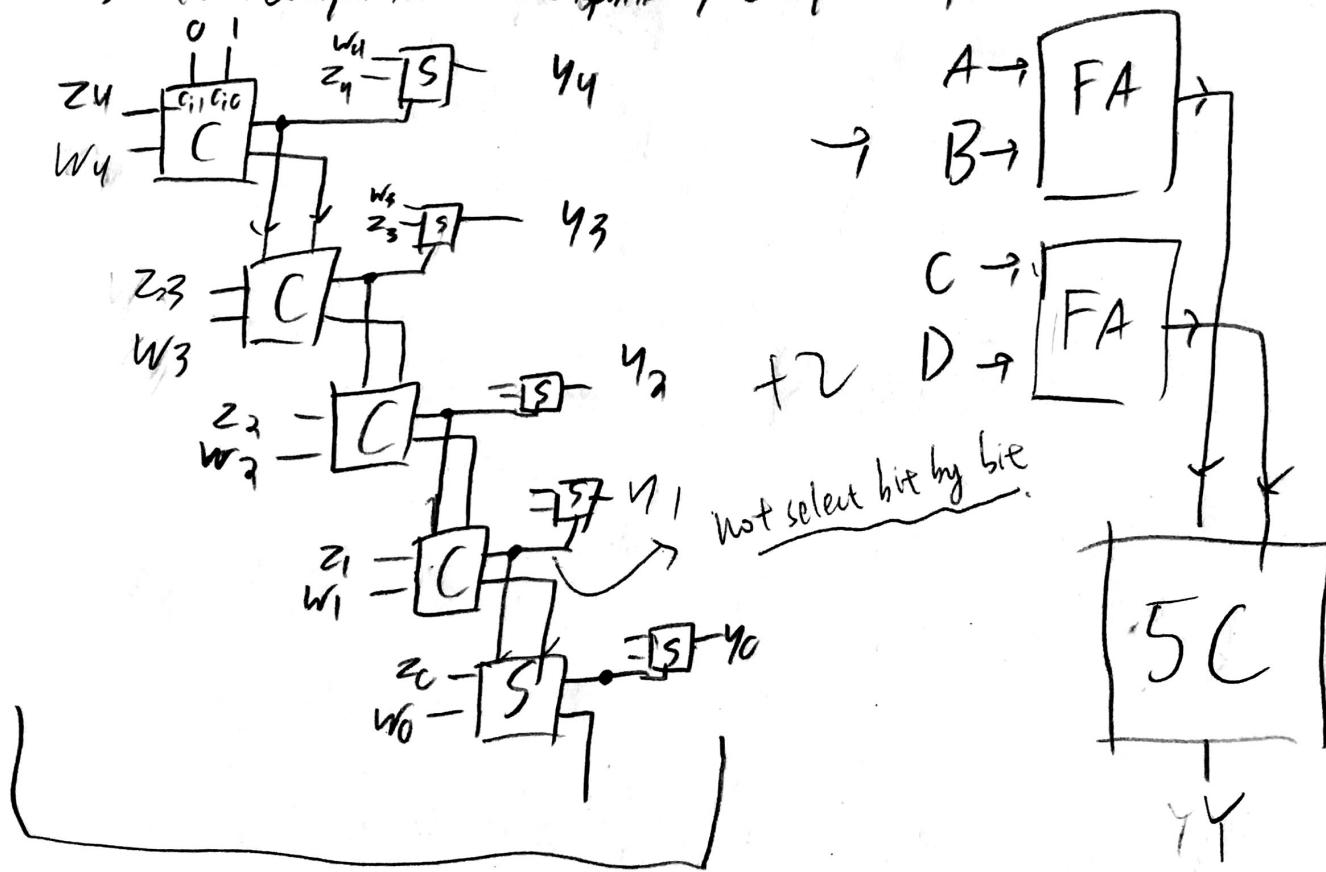
$$SC \quad \begin{matrix} Y \\ Z \\ W \end{matrix} = 5C \rightarrow Y \quad Y = \text{Max}(Z, W) = \text{Max}(A+B, C+D)$$
