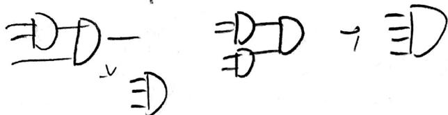
4 input OR gate using 2-input OR gate:
