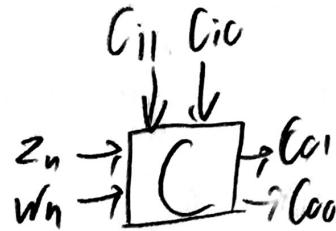
$$\begin{aligned} C_{out} = 0 & \text{ if } Z_n > W_n \\ & \text{if } Z_n = W_n \\ & 1 \text{ if } Z_n < W_n \end{aligned}$$
