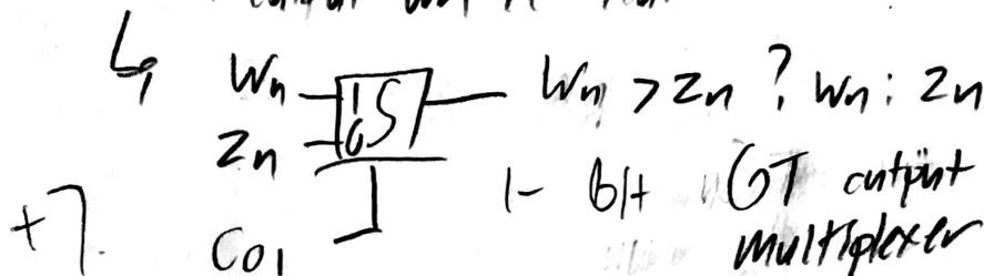
5-bit Comparator and outputs  $\rightarrow$  Outputs  $Y = \text{Max}(Z, W)$
