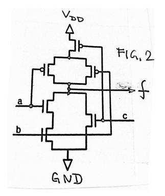
Figure 2: CMOS Circuitk
