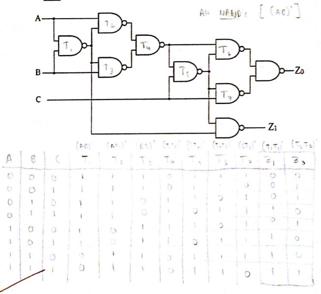
b) From a high-level description, what <u>mathematical</u> function is the network performing? Do <u>not</u> state your answer simply as when the output equals 1 such as: "z<sub>1</sub> = 1 when A = ... and B = ... and C = ...", but give a clear descriptive answer.
