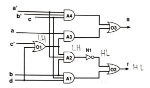
Part(a) Assume that negated variables are available. Find the *critical path* of the above network by listing its gates along the path, starting at the inputs:
