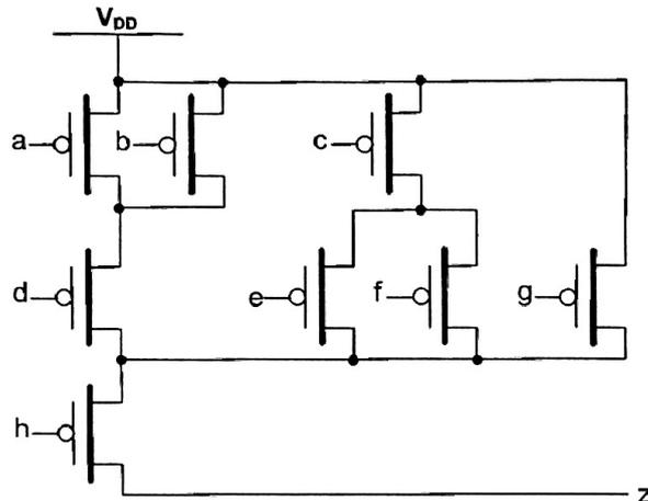
1. (5 points) Write the expression for the pull-up network. From this, derive the expression for the pull-down network using switching algebra. Make sure the inverters are on the correct variables.
