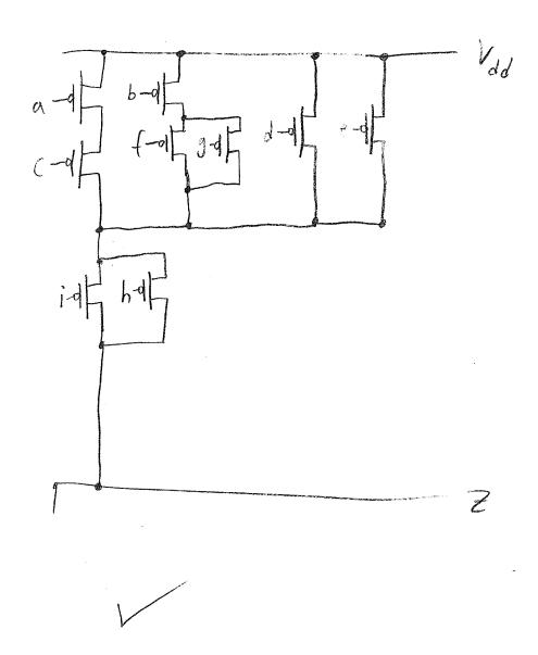
2. (7 points) Draw a CMOS network that implements f(x,y) = xy' + x'y (2-input XOR). x' and y' are not available as inputs. Do not use transmission gates. How many transistors does your solution have? OPTIONAL: If you find another solution with fewer transistors, you get 3 extra points. Show your reduced design and explain why it works.
