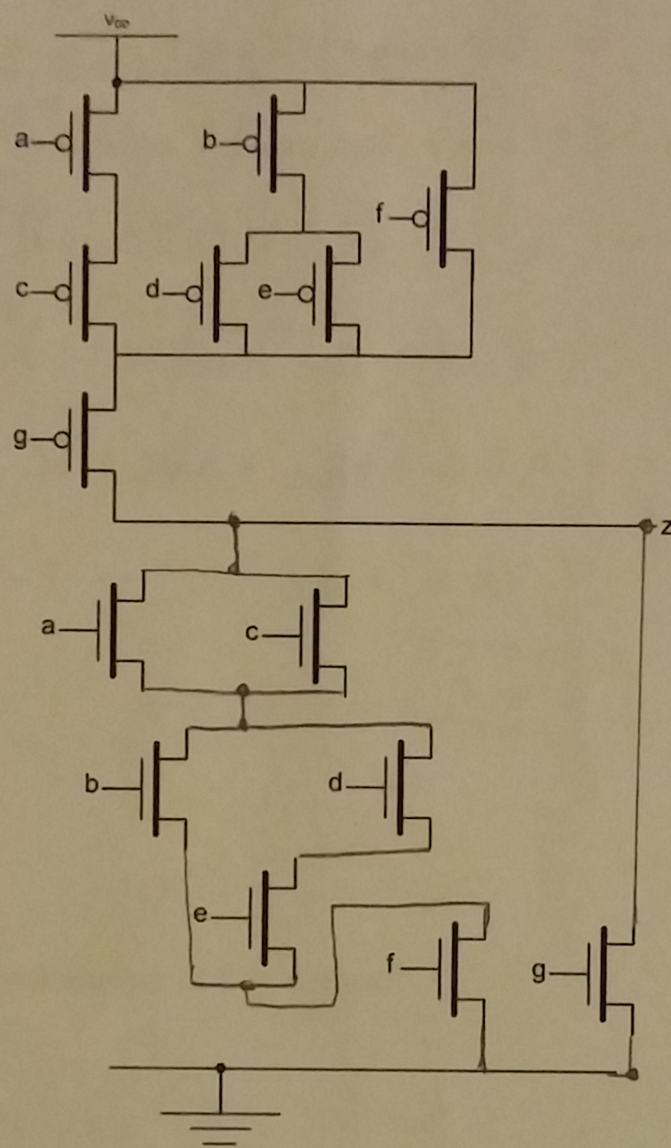
1. (10 points) Write the expression for the pull-up network. From this, derive the expression for the pull-down network using switching algebra.
