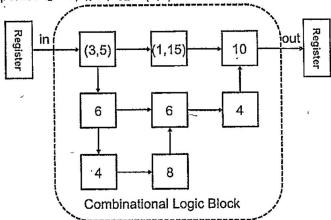
(a) (4) Determine the contamination and propagation delay of the combinational logic block.
