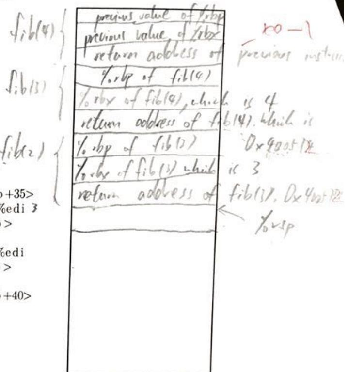
1. This function calls itself recursively. Imagine in gdb we put a breakpoint on line 0x40056d, then call fib(4). Furthermore we hit continue two more times in gdb, so that the stack frames of fib(4), fib(3), and fib(2) are all on the stack. Draw the contents of the stack in the box above, and be sure to indicate the stack pointer. Draw everything you know about the stack! If you know what the value is, write the value, otherwise indicate what it is. (10 pts)
