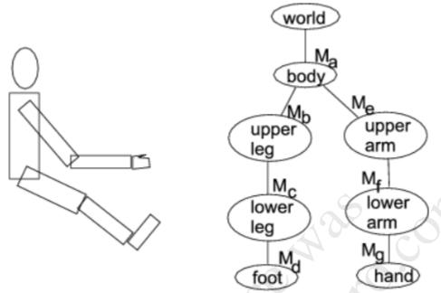
(7 pts) Determine an expression for the composite transformation matrix that would be used to draw the hand, i.e., that takes a point from the hand coordinate frame to the world coordinate frame.
