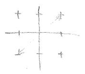
The maximal margin y is the greatest distance between a positive and negative example in the dataset. In the OR dataset it would be the distance between (-1,-1) and (1,1) which is  $\sqrt{(1+1)^2 + (1+1)^2} = \sqrt{8} = 2\sqrt{2}$ . . .
