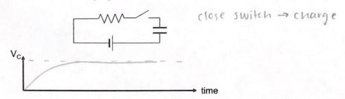
6. The capacitor in the circuit shown is charged. Sketch the voltage drop across the resistor as a function of time after you close the switch.
