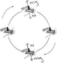
• 7a) Solve for the normal force the carpet exerts on Jazmine at the bottom of the vertical loop.
