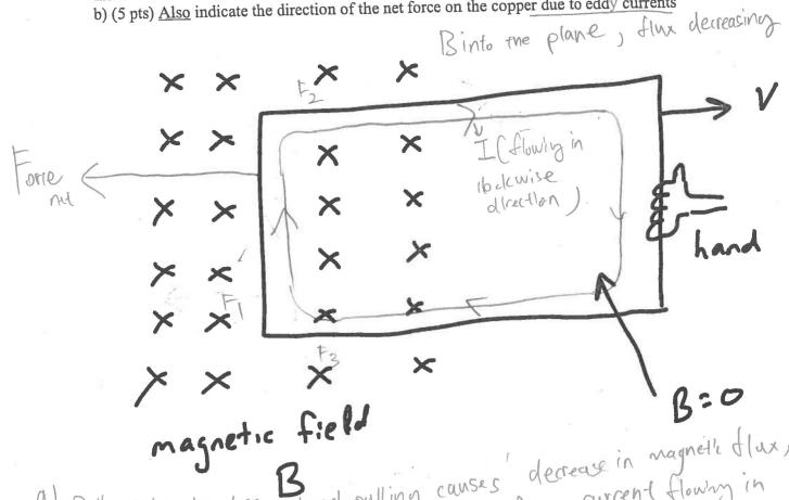
a) Bedrused into the plane, hand pulling causes decrease in magnetle flowing in induced emf to proverte charge in magnetle flow, current flowing in clockwise direction as shown in the diagram.
