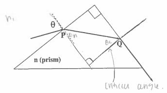
a) Determine an expression for the index of refraction of the prism,  $n_{prism}$ , in terms of the angle of incidence  $\theta$ . Your expression should not depend on angles other than the angle of incidence. For an angle of incidence of  $60^{\circ}$ , what must the index of refraction be for the light ray to take this path?
