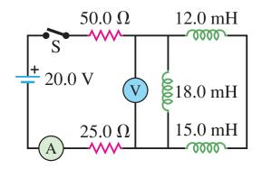
In the circuit shown in the figure, the switch has been open for a long time and is suddenly closed. Neither the battery nor the inductors have any appreciable resistance.
