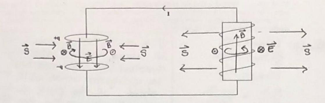
A circular parallel-plate capacitor of plate area A and plate separation d is connected across a solenoidal inductor of radius a, length x and n turns per unit length. At the instant under consideration, the capacitor has a charge q (polarity shown above), and a current I is flowing through the circuit in the direction shown. We do not know the instantaneous rate at which the current is changing, but it may be possible to infer that from the other information we know.
