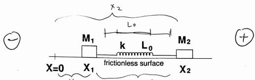
1) A pair of masses,  $M_1$  and  $M_2$  are joined by a spring of constant k and natural (unstretched) length  $L_0$ .
