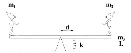
Consider the child's toy shown above. A uniform rod, of mass  $m_3$  and length L is attached to a pivot that passes through its center of mass. Small clowns, of mass  $m_1$  and  $m_2$  are glued on opposite ends of the rod. A spring, of constant k, is mounted vertically between the base of the toy and the rod, a distance d from the rod's center of mass. The spring is not extended or compressed when the rod is horizontal. The rod is displaced slightly, and the system begins to rock...
