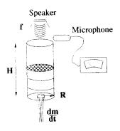
Consider the apparatus shown above... Sound (of frequency is emitted by a speaker into a tube of radius (R) and height (H). A microphone, placed near the open end of the tube, is used to monitor the intensity of the sound that is re-radiated from the tube. There is liquid (of volume mass density  $\rho$ ) partially filling the tube, and it is leaking from a hole (of negligible area) in the bottom of the tube at a rate  $\frac{dm}{dt}$  (m is mass).
