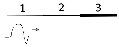
i. A wave pulse, drawn above, is traveling on string 1, approaching the knot between string 1 and 2. Draw the reflected pulse and the pulse which is transmitted onto string 2. In your drawing, pay attention to whether or not the pulses are inverted/upright but also to the overall shape of the pulse – e.g. are the reflected/transmitted pulses stretched out or compressed relative to the incident?
