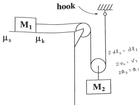
Consider the apparatus shown above. The coefficients of friction between block one and the table are both known, as are the masses  $M_1$  and  $M_2$ .
