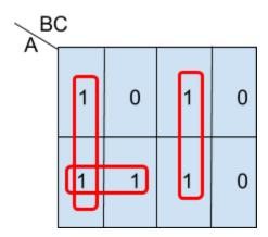
B. Show a combinational circuit that implements F using only inverters and NAND gates.
