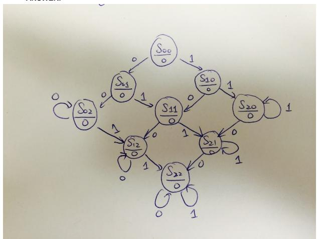
C. Design a state transition diagram for a Moore state machine that takes one input A and has one output X, which should be 1 if, and only if, the last four values of A have been either 1011, 1001, or 0100 (the left most bit represents the oldest value among the four).
