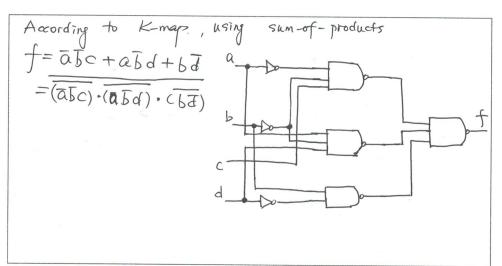
(c) (5 points) Show a combinational circuit that implements f using minimum number of inverters and NOR gates only. The maximum number of inputs per gate is less than 4.
