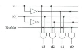
on E turns decoder off, setting all  $d_i$ s to 0. Value 1 on E turns decoder on. Design a combinational circuit that converts a 3-bit sign-and-magnitude number, a, into a 3-bit one's complement number, b. You are allowed to use any number and any combination of the following building blocks:
