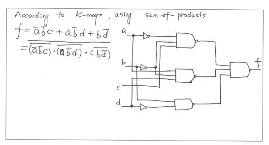
(c) (5 points) Show a combinational circuit that implements f using minimum number of inverters and NOR gates only. The maximum number of inputs per gate is less than 4.
