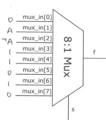
4. (10 points) Design a combinational network that has a three-bit input x representing the digits 0 to 7, and a three-bit output y representing the same set of integers. The function of the system is  $y = (x+3) \mod 8$ . You may use any building blocks and gates you have learnt.
