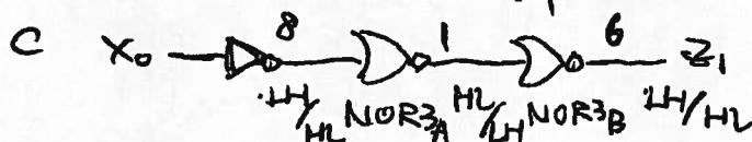
$$t_{PLH}(x_0, z_1) = t_{PLH}(\text{NOR}_3^B) + t_{PHL}(\text{NOR}_3^A) + t_{PLH}(\text{NOT})$$
